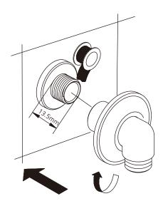
Before installation, please note that the length of the connecting adaptor that protrudes out of the wall should be 0.53" (13.5mm) long. Apply pipe tape on the end threads of the connecting adaptor. Install the wall outlet to the connecting adaptor tightly, then slide the decorative escutcheon over the wall outlet and push against the wall.
